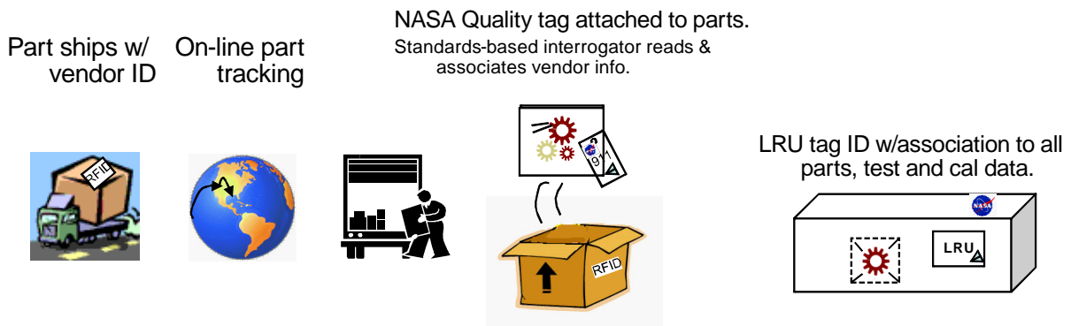
Figure 3-2: RFID Ground-to-Line Replacement Unit Concept
