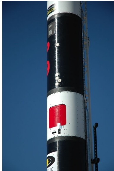
Figure D-3: Passive Temperature RFID/Sensor Tags on Rocket Fuel Tank
